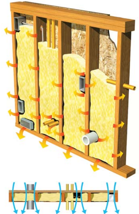
Air escapes easily through and around fibrous batt insulation, decreasing insulation efficiency and trapping dirt and moisture in the fibers.
