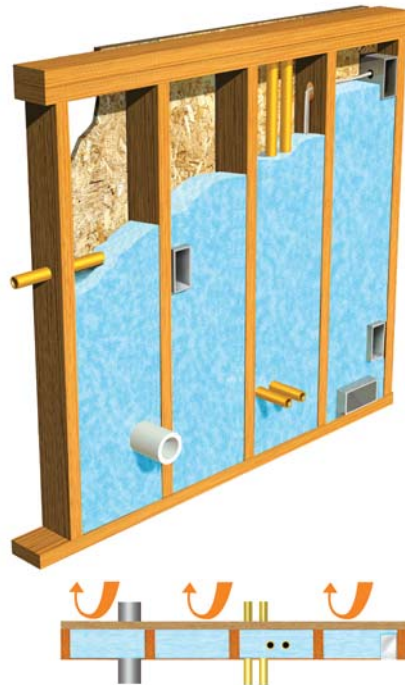
STYROFOAM™ Brand SPF Insulation provides an edge-to-edge air seal, effectively blocking random air leakage and moisture intrusion.
